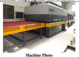
State of Art Horizontal Tempering Line (LANDGLASS) is loaded with full Convection furnace offering wide range of high performance glass (ST, ET, KT & SKN Series of SAINT GOBAIN) and other equivalent glasses producers like AIS and GUARDIAN. We use most energy efficient tempering technologies (30 Kw Blower for 10 to 19 mm full tempered glass) with fully Automatic CNC controlled interface.
