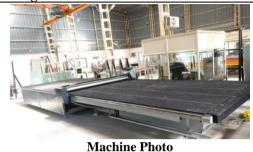
CNC Glass Cutting Line (LISEC) relates to fully mechanized glass loading system for achieving the most accurate (0.2mm Accuracy) and fastest cutting speed of 150 Sq. per Meter per hour which is the best in the industries.
